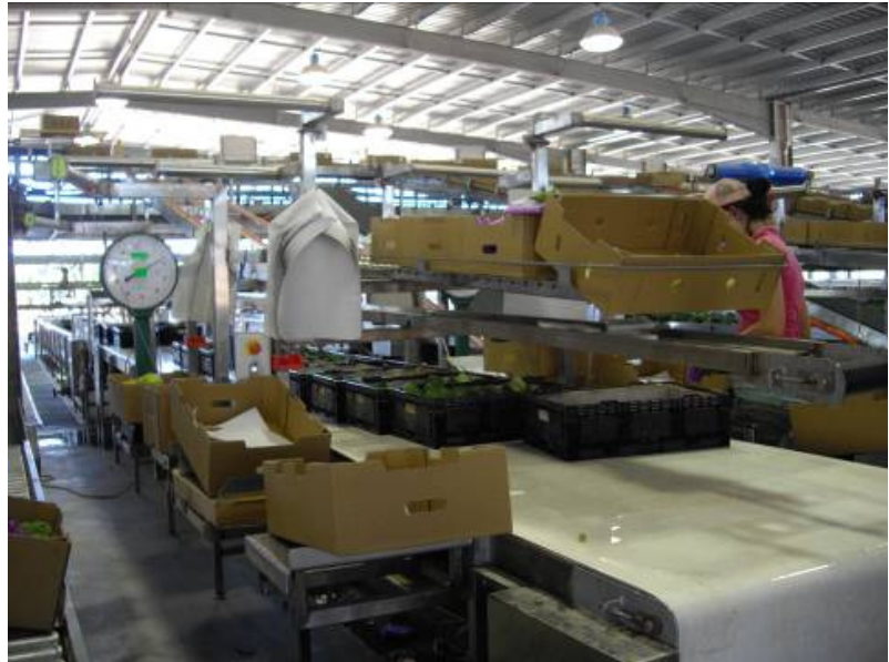
Figure 10. Single line grading system packing straight in the carton and minimising handling
