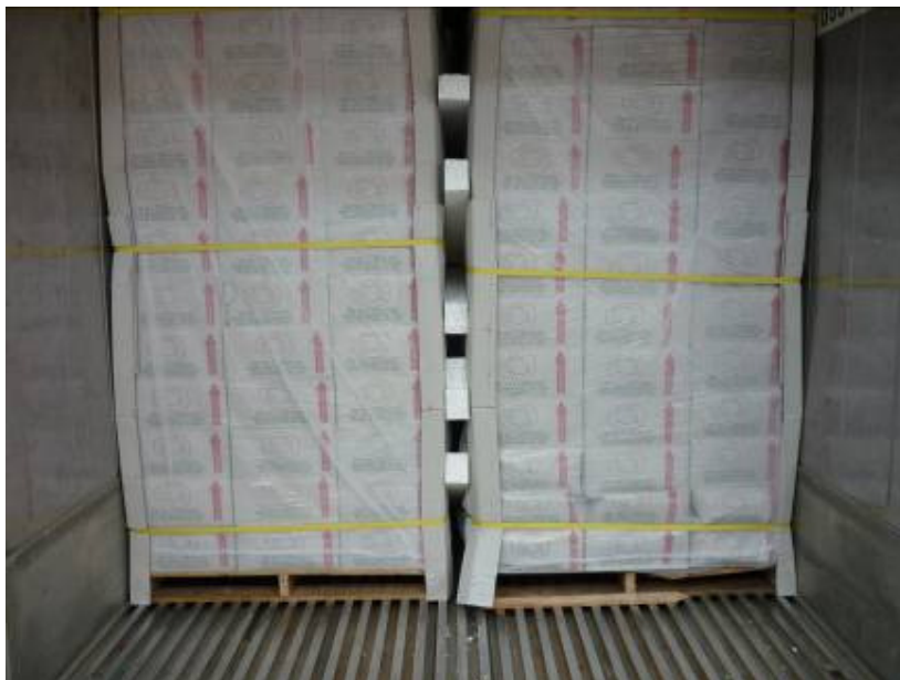
Figure Eight: Comparison of cartons with extra collar (left) to standard carton.
