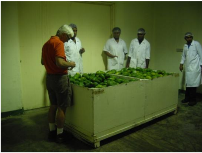
Pre-cooling in NWC cold room immediately after completion of HTFA treatment.
