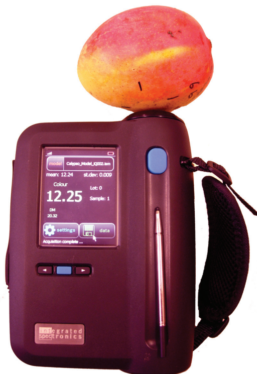
Plate 15. Hand held NIR unit (Nirvana), in position on a labelled piece of fruit
