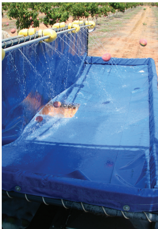
Plate 20. Harvest aid with a vertical tarpaulin to reduce the momentum of thrown fruit
