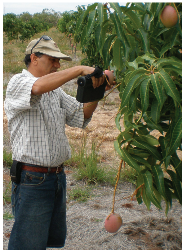
Plate 14. Hand held NIRS unit (Nirvana) in use on a Calypso™ mango tree
