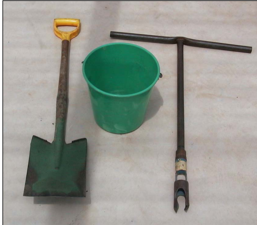
Figure 3. Basic equipment is all that is required to collect a soil sample. The auger shown on the right is useful but not essential. A meaningful sample can be collected with a plastic bucket and a spade or shovel.
